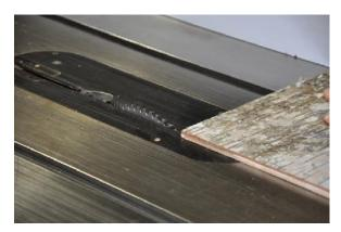
If your panel has to be site cut, ensure that you take the same precautions as with cutting any other finish veneer panel. Use proper cutting blades with the appropriate number of teeth as to minimize chipping and flaking of the bark veneers.
